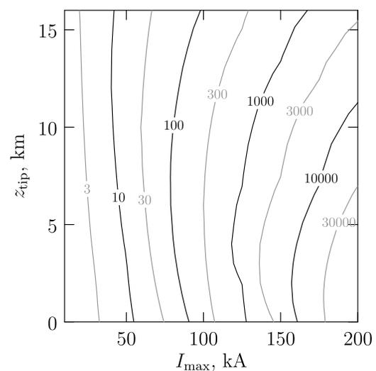
**Figure 3.** Contour plot of the altitude and current pulse dependence of the maximum avalanche growth of populations of runaway electrons injected near the tip of a 1 km lightning leader channel. Contour labels indicate the avalanche growth factor  $\mathcal{M}$ .
