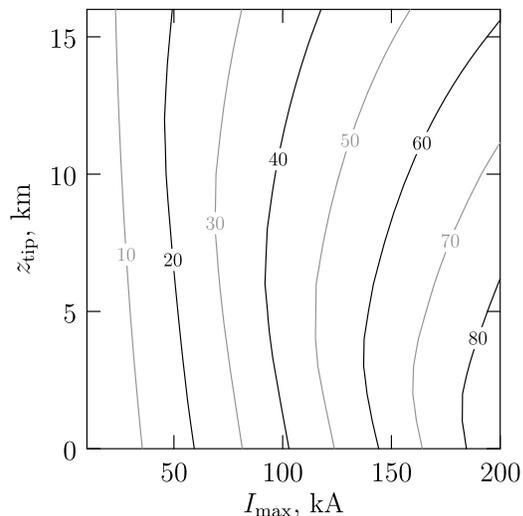
**Figure 2.** Contour plot of the altitude and current pulse dependence of the maximum possible energy gain for electrons injected near the tip of a 1 km lightning leader channel. Contour labels indicate energy gain in MeV.
