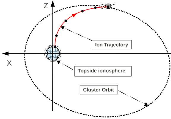
**Figure 1.** Schematic diagram showing the tracing technique. For every cold ion recorded, its acceleration along the magnetic field line and convection velocity can be calculated to trace the cold ion along its trajectory, all the way back to topside ionosphere. The final landing point in the ionosphere is defined as the source region.
