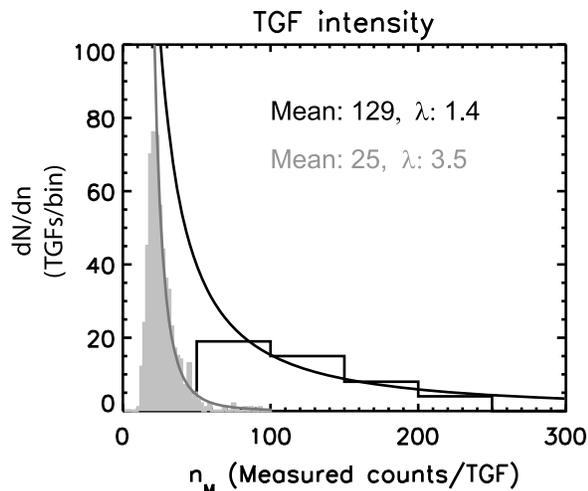
**Figure 1.** The fluence distributions of TGFs measured by RHESSI (grey histogram) and Fermi (black histogram). Power functions are fitted to both distributions. The average values for Fermi are for TGF pulses, defined as counts in the central 50% of duration.
