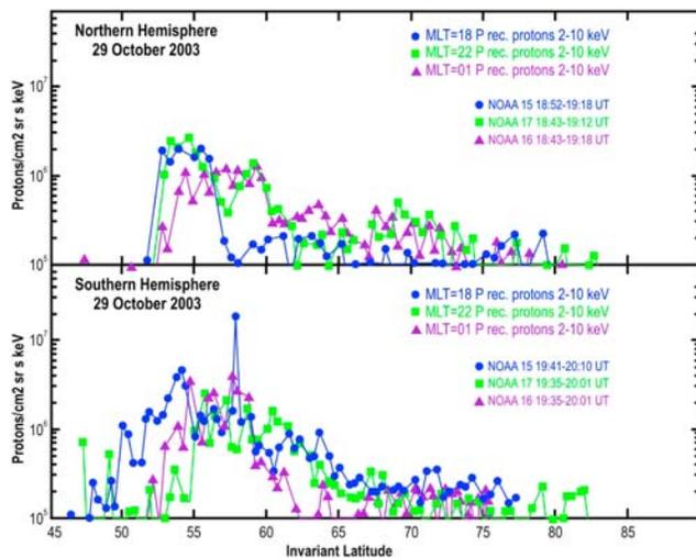
**Figure 1.** NOAA 15, 16, and 17 Total Energy Detector (TED) measurements of ion precipitation in the energy range (2–10) keV are plotted versus invariant latitude at 3 local times in the northern and southern hemisphere.
