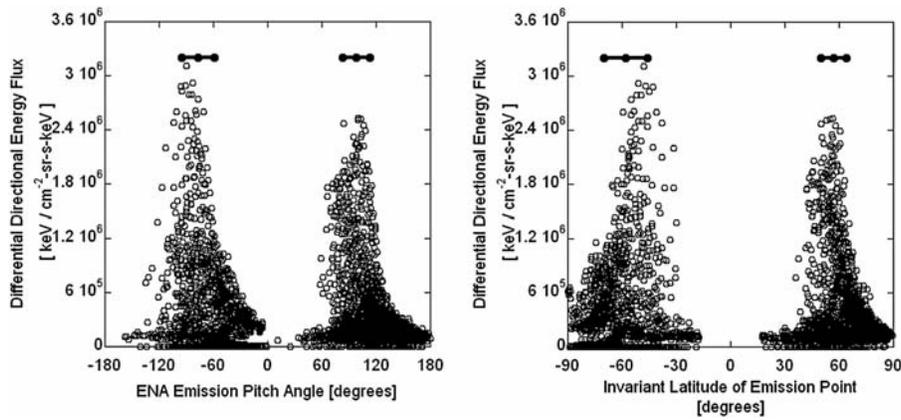
**Figure 3.** Differential directional ENA flux in the energy range (2–5) keV recorded in a MENA image pixel is plotted versus the estimated emission (left) Pitch Angle and (right) Invariant Latitude of the emission source associated with that pixel. Mean values, weighted by ENA flux, and standard deviations for the Pitch Angle and Invariant Latitude distributions are also shown.
