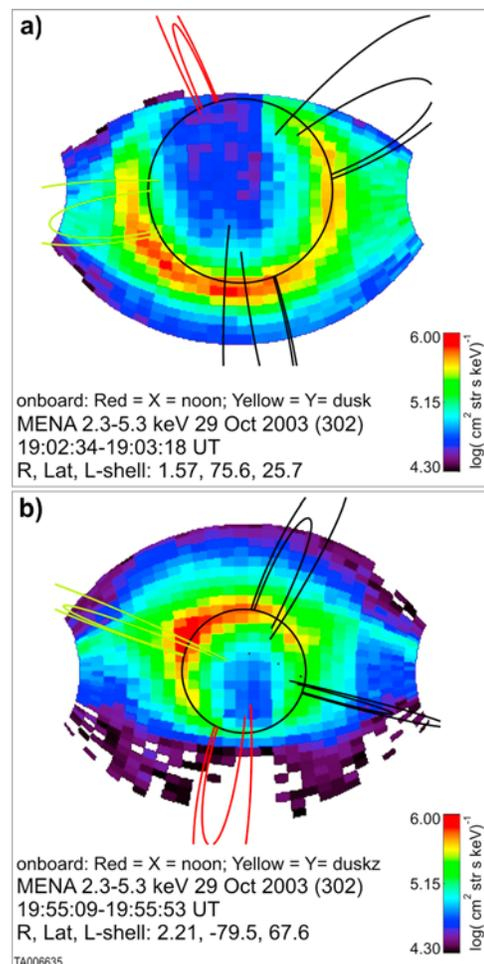
**Figure 2.** (a and b) Two MENA flux images in the energy range (2–5) keV/nucleon are presented. Each is annotated with geomagnetic dipole field lines at MLT = 0, 6, 12 (red), and 18 (yellow) hours, at  $L = 4$  and 8. The circle at the center of each image indicates Earth limb. The common color bar at right provides logarithmic scaling of the differential directional ENA flux at the observation point. The image in Figure 2b was obtained from above the northern (southern) polar region.
