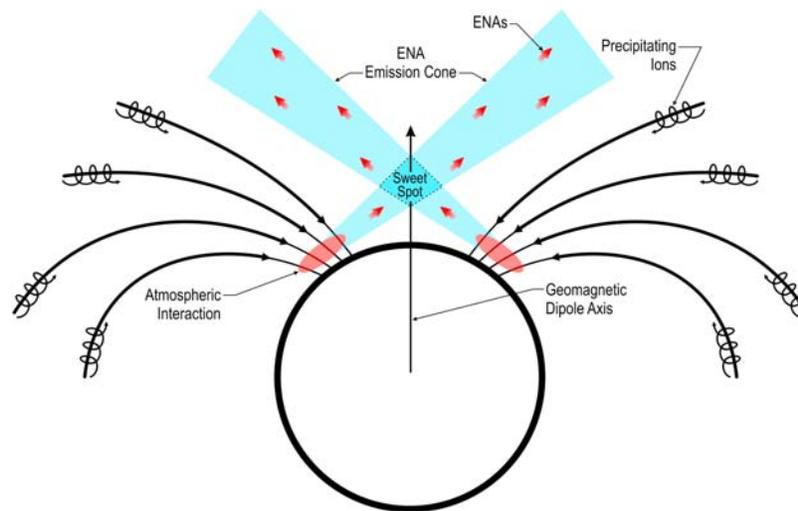
**Figure 4.** Concept of an ENA emission cone, emanating from the footpoints of the ring-current ion precipitation, is illustrated.
