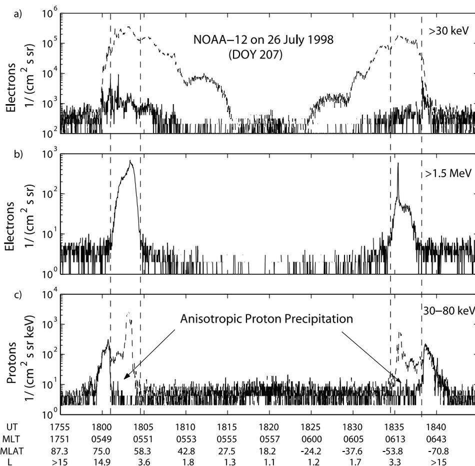
**Figure 2.** Particle data from a pole-to-pole morning side orbit by NOAA-12 on 26 July 1998. From the top is shown electrons  $>30$  keV, from both the 0deg (solid line) and 90deg (dashed line) MEPED detectors, electrons  $>1.5$  MeV measured by the dome detector, and 30–80 keV protons, measured by the 0deg (solid line) and 90deg (dashed line) MEPED detectors. The dashed vertical lines delimit the anisotropic proton zone.
