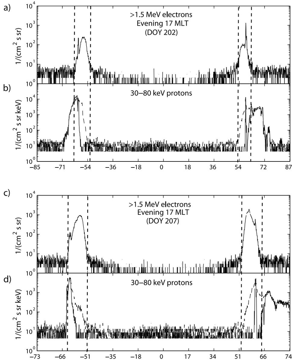
**Figure 4.** Particle data from NOAA-12 on 21 and 26 July 1998. The figure exhibits electrons  $>1.5$  MeV and protons 30–80 keV, from the 90deg (dashed line) and 0deg detectors (a and b) from an eveningside pole-to-pole orbit on 21 July (1215–1305 UT) and (c and d) from an eveningside pole-to-pole orbit on 26 July (0700–0751 UT).
