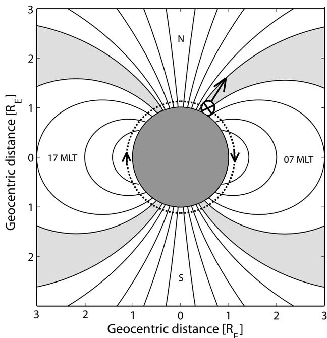
**Figure 1.** NOAA-12's orbit relating to the Earth's magnetic field and the direction of the vertical and horizontal detectors. At high latitudes ( $>50^\circ$ ) the vertical detector looks approximately along the magnetic field and around the equator it looks normal to the magnetic field. The horizontal detector, however, looks normal to the magnetic field during the whole orbit.
