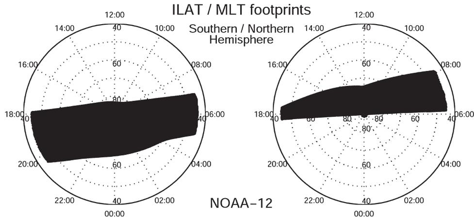
**Figure 1.** ILAT/MLAT footprint of the NOAA-12 spacecraft. Southern Hemisphere to the left, and Northern Hemisphere to the right.
