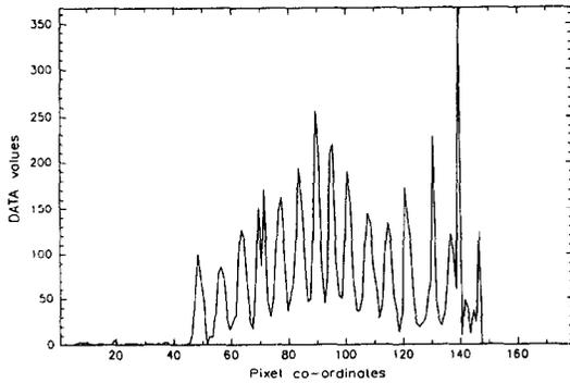
Fig. 8. Response function of CsI(Tl) ladder illuminated with 22 keV -rays.
