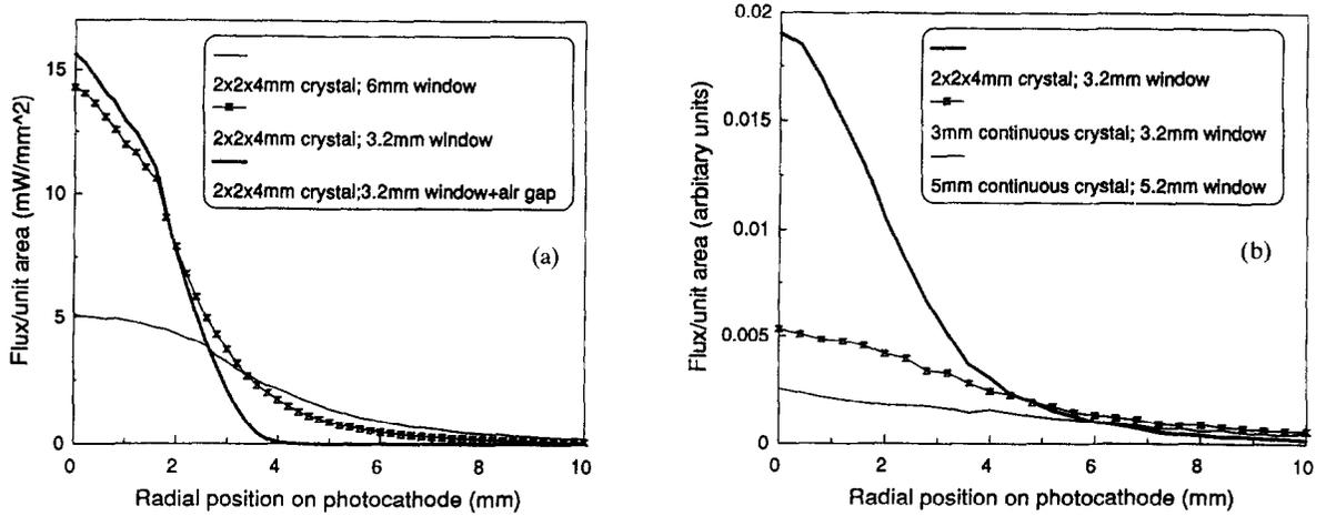
Fig. 3. (a) Optical Monte-Carlo simulations illustrating the effect of glass window thickness on light spread. (b) Optical Monte-Carlo simulations illustrating the effect of crystal dimensions on light spread.
