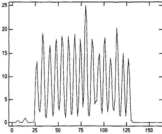
Fig. 7. 2 mm crystals illuminated by 122 keV ( $^{57}\text{Co}$ ) with multi-wire readout. Detector response is 1.2 mm FWHM.
