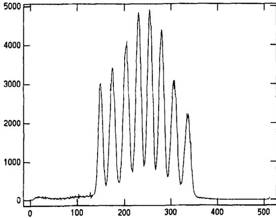
Fig. 4. 3 mm crystals illuminated by 122 keV ( $^{57}\text{Co}$ ) with conventional readout. Detector response is 2.1 mm FWHM.
