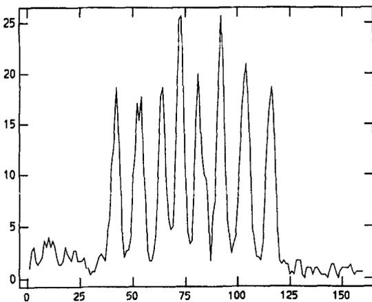
Fig. 5. 3 mm crystals illuminated by 122 keV ( $^{57}\text{Co}$ ) with multi-wire readout. Detector response is 1.5 mm FWHM.
