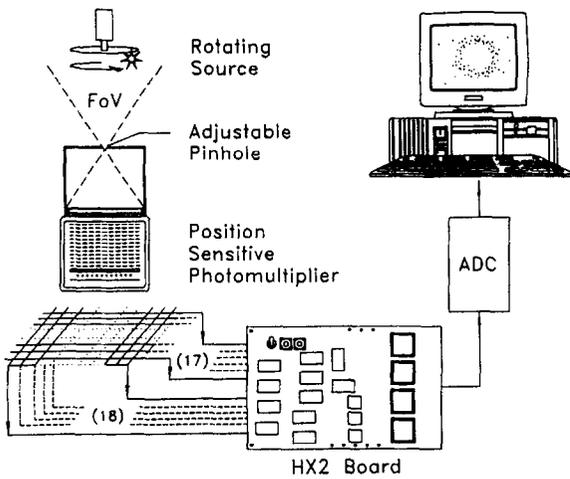
Fig. 1. Arrangement of rotating X-ray source and imager.
