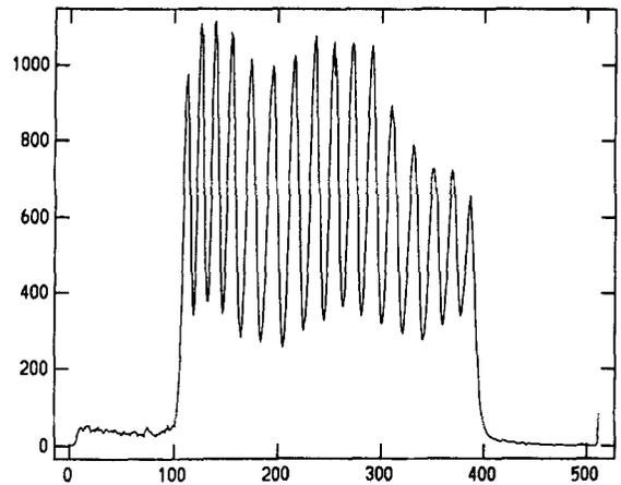
Fig. 6. 2 mm crystals illuminated by 122 keV ( $^{57}\text{Co}$ ) with conventional readout. Detector response is 1.5 mm FWHM.
